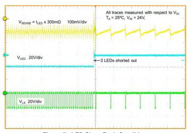
Figure 7 LED Short Fault Condition
