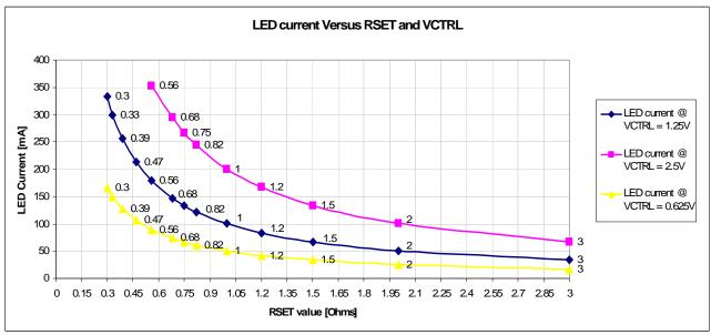
Figure 4 LED Current Setting vs.  $R_{\text{SET}}$  and  $V_{\text{CTRL}}$
