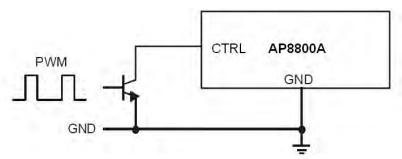
Figure 6 Open Collector PWM Dimming Circuit
