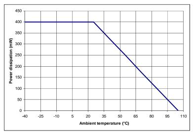
Figure 8 Derating Curve
